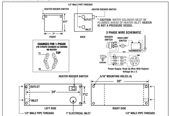
The CMA-Temp-Sure™ option assures a continuous supply of 140°F hot water resulting in excellent dishmachine performance. The heater is custom-designed for fill and dump CMA single tank dishwashers as a factory added option or an infield add-on. The heater will also fit most competitor's single tank dishmachines.
