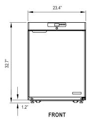
\*For Built-In Applications: Allow 1.2" (30mm) at top for stainless steel louvered vent (supplied with unit).
